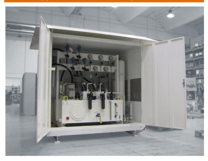
**SUPPLY**: power unit with cabinet for diverter damper control in combined cycle power plants
