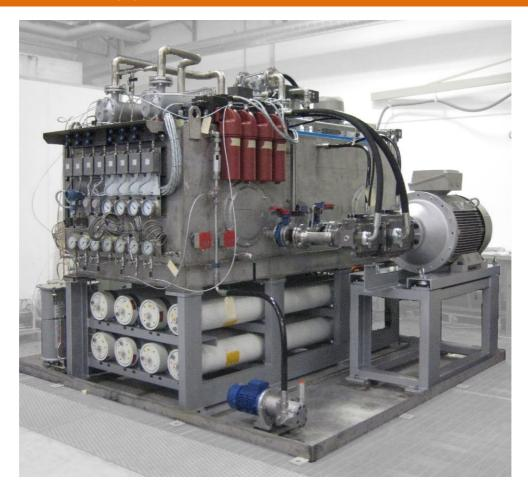
**SUPPLY**: Hydraulic system for the control of a 650 MW steam turbine (nuclear power station)
