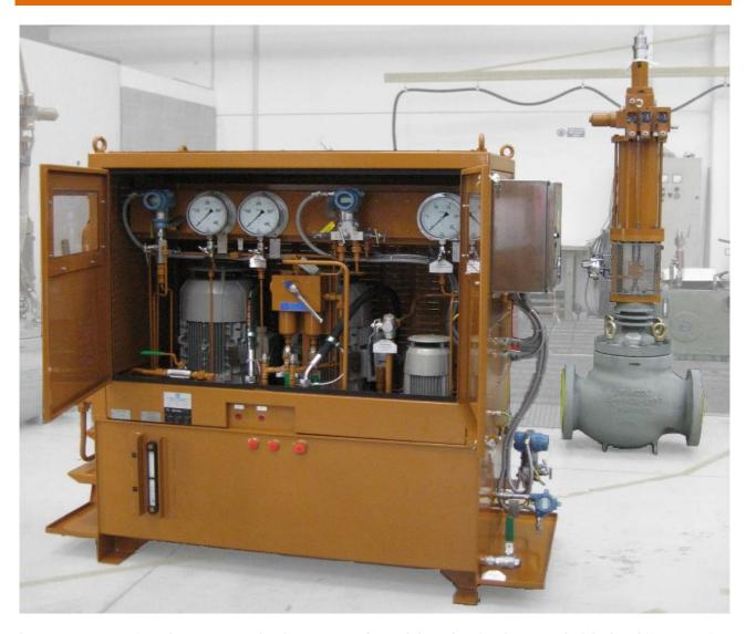
**SUPPLY**: Power unit and 2 groups made of actuator and 10" globe valve for the control of ORC turbine operation mode (from connected to the grid to island mode and viceversa).
