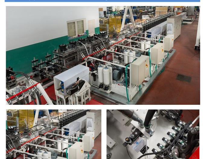
SUPPLY: Power units and cylinders for metal roll forming lines
