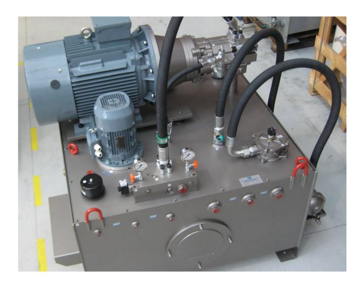
**SUPPLY**: Hydraulic power unit for laser tube cutting machines
