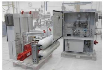
SUPPLY: Power units for the control of the actuator and of the sectioning valves
