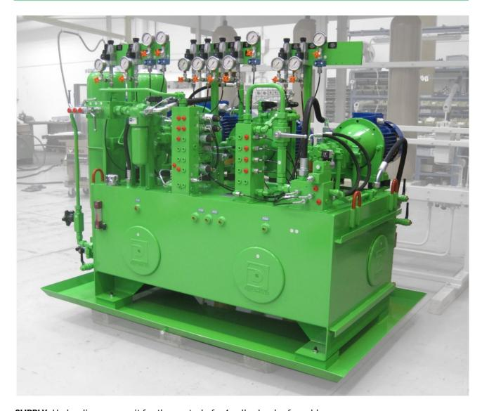
**SUPPLY**: Hydraulic power unit for the control of a 4-roll calender for rubber
