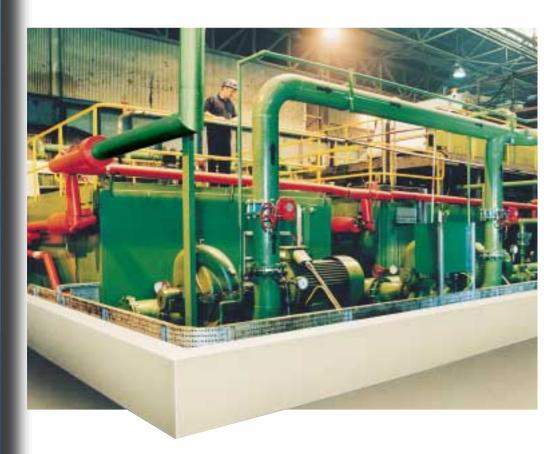
Systems custom designed with the coolant flow rate, cleanliness and heat dissipation meeting the specific requirements of the rolling mill.
