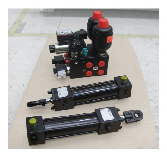
SUPPLY: hydraulic control system for gyroscope stabilizer
